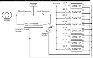
The unit allows the synchronization scheme defined in the above picture. The application is made with standard units and standard software, without extra cost. No additional parts are needed.
